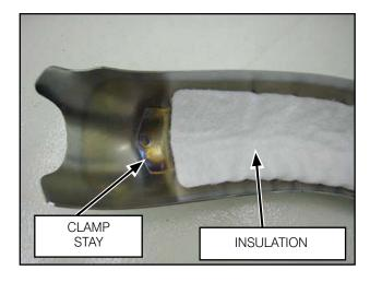
Reinstall the exhaust pipe cover with installed insulation.
