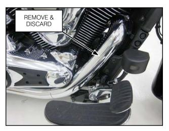
• Install exhaust pipe cover provided in the kit.
