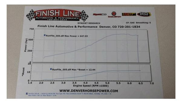
These results are on a 2015 1LE car with the LS3, 12psi of boost, 12\* of timing, our Premium Bundle Package with fueling pack #1. 647 rwhp, 620 rwtq. Comp Billet 7875, 3bb turbo with larger 1.15 a/r housing option.
