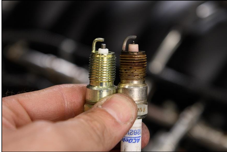
New ACCEL Spark plugs compared to the OEM projected tip plugs
