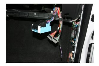
Install the antenna to the right of the mirror and route the wire down the passenger A-pillar to the underside of the dash. Pass the 16-Pin, Antenna and Drone Cable (if used) over the heater brace. Run the 3 wires for the rear of the CJB behind the metal bracket so they will not get pinched when the CJB is reinstalled:
