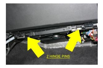
The trickiest part of the installation is removing Central Junction Box (CJB), which is the fuse block behind the glove compartment. But when removed, you will have access to all the necessary wires.
