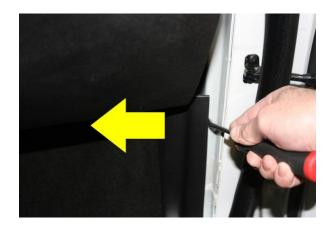
Remove the plastic panel under the dash. Unplug the light:
