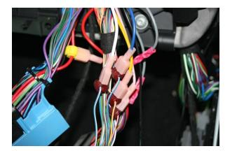
Here are the Orange and Green connectors that you had to blindly disconnect from the back of the CJB. Again, be sure to run the 3 wires behind the black metal bracket so they do not get pinched upon reassembly:
