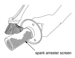
4. Install the spark arrester and the gasket in the muffler, and tighten the bolts to the specified torque:
