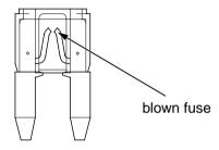
Check all the fuses before looking elsewhere for another possible cause of the problem. Replace any blown fuses and check component operation.
