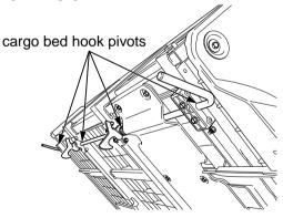
Lubricate the cargo bed strikers as shown in the following illustration. Lift the cargo bed (page 44).
