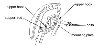
To return the seat-back to a more rearward position, follow the general instructions above, setting the lower hooks on the support rod and using the lower bolt holes.
