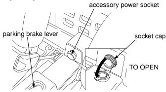
To use the accessory power socket, the engine must be on and idling.
