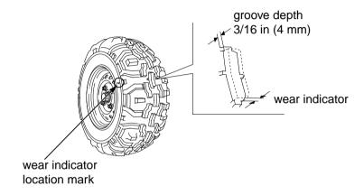
To check the condition of a tire tread, measure the groove depth in the center of the tire, or check the wear indicator.
