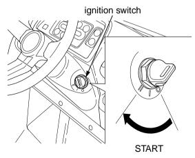
To stop the engine, turn the ignition switch to the OFF (O) position. Remember to apply the parking brake and remove the key if you plan to leave the vehicle.
