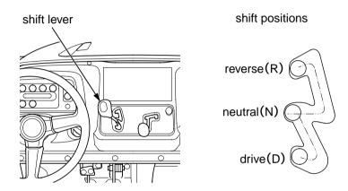
You should move the shift lever only when the vehicle is stopped with your foot on the brake pedal and with the engine idling. Use a firm motion to select the appropriate gear. Have your vehicle checked by a Honda dealer if you experience any shifting problems.
