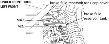
It should be between the MIN and MAX level marks. If the level is at or below the MIN level mark, check the brake pads for wear (page 138).
