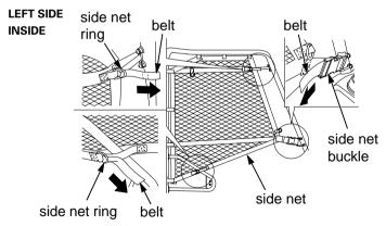
Be sure the side nets are properly latched before driving your Honda MUV, and never remove a side net.
