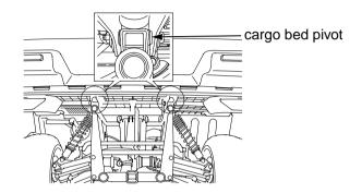
Lubricate the cargo bed hook pivots as shown in the following illustration.
