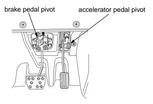
Lubricate the parking brake pivot as shown in the following illustration. Remove the center panel (page 128).
