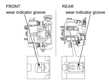
Always inspect both pads in both the right and left brake calipers.
