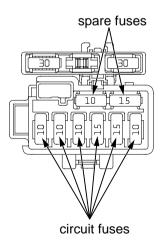
If you do not have a spare fuse and you cannot drive the Honda MUV without fixing the problem, take a fuse of the same rating or a lower rating from one of the other circuits that you can do without temporarily.
