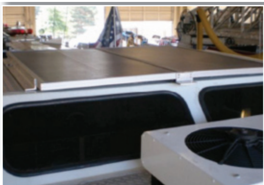
PV Installation on a Fire Truck in Johnson County, Kansas
