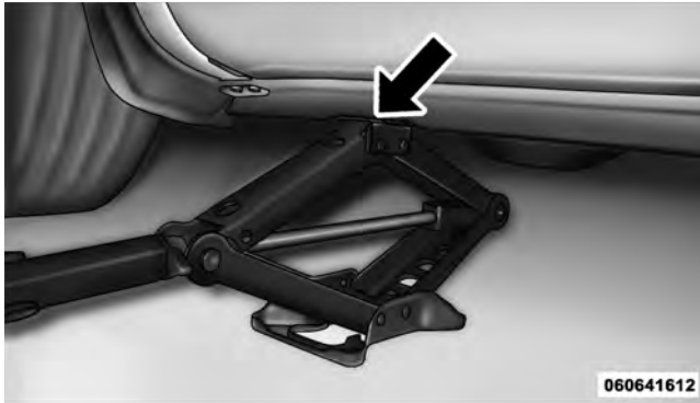
Front Jacking Location
