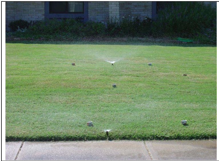
Figure 1. Using cat foot cans to audit irrigation system in home lawn.
