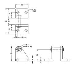
Rod Clevis Bimba Part Number **D-231-3**  Rear Pivot Bracket Bimba Part Number **D-620**
