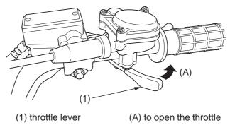
The throttle controls engine rpm (speed). To increase engine rpm, press the throttle lever (1) with your thumb. To reduce engine rpm, release pressure on the throttle lever. The throttle will automatically return to the closed position (engine idle) when you remove your thumb.
