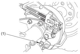
(1) rear brake drain bolt
