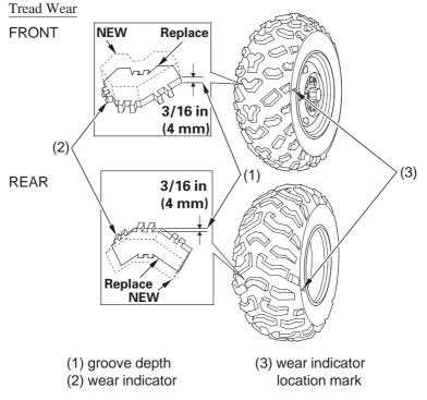
To check the condition of a tire tread, measure the groove depth (1) in the center of the tire, or check the wear indicator (2).
