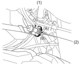
(1) rear brakelight switch(2) adjusting nut
