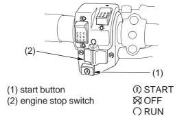
The start button (1) is used for starting the engine. Pushing the button in starts the engine. See *Starting Procedure*, page 61.
