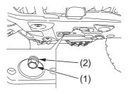
(1) engine oil drain plug (2) sealing washer
