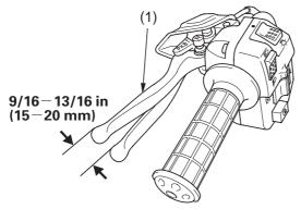
(1) rear brake lever/parking brake lever
