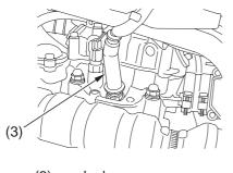
(3) spark plug cap(4) center electrode
