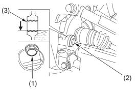
(1) oil drain plug(2) oil fill cap
