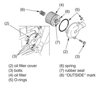
6. Reinstall the oil filter cover, making sure the bolts are tightened to the specified torque:
