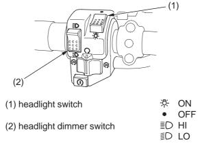
The headlight switch (1) is used to turn the headlight ON (  $\mbox{\ensuremath{\ensuremath{\otimes}}}$  ) or OFF (  $\mbox{\ensuremath{\circ}}$  ). To operate, turn the switch to ON (  $\mbox{\ensuremath{\ensuremath{\otimes}}}$  ) or OFF (  $\mbox{\ensuremath{\circ}}$  ).
