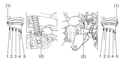
(1) spring pre-load adjuster(2) pin spanner
