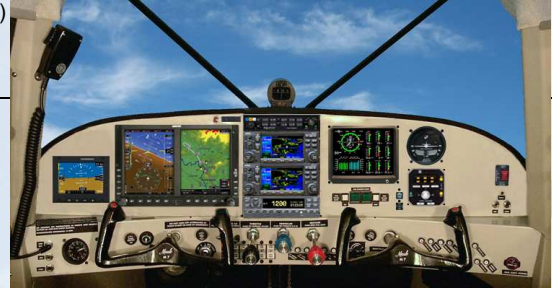
G500 FDS shown with optional L-3 Trilogy ESIS, S-Tec 50 Autopilot, and IFR-FortyW with Second Garmin GNS430
