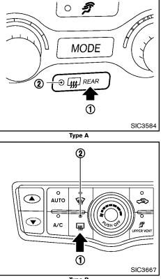
To defog/defrost the rear window glass and outside mirrors (if so equipped), start the engine and push the switch ① on. The indicator light ② will come on. Push the switch again to turn the defroster off.
