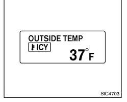
Outside air temperature (ICY - °F or °C) The outside air temperature is displayed in °F or °C in the range of -22 to 140°F (-30 to 60°C).
