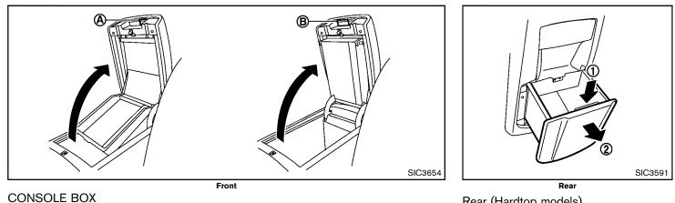
Rear (Hardtop models) To open, push the knob ① and pull out ②.
