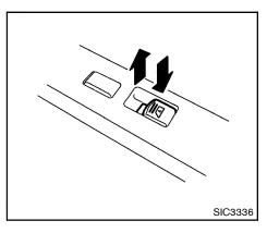
Passenger side power window switch The passenger side switch will open or close only the corresponding window. To open or close the window, push down or pull up the switch and hold it.
