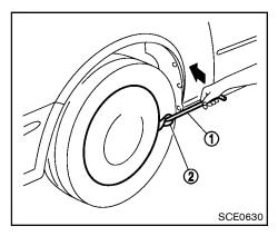
Removing wheel cover (if so equipped)
