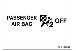
7. If the booster seat is installed in the front passenger seat, place the ignition switch in the ON position. The front passenger air bag status light == n- may or may not illuminate depending on the size of the child and the type of booster seat used. See "Front passenger air bag and status light" later in this section.
