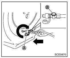
Remove the protective cap (A) of the hose and screw the hose securely onto the tire valve. Make sure that the pressure release valve (B) is securely tightened. Make sure that the air compressor switch is in the OFF (O) position, and then insert its power plug into the power outlet in the vehicle.
