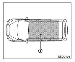
Operating range for engine start function The Intelligent Key functions can only be used for starting the engine when the Intelligent Key is within the specified operating range 1.
