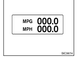
Average fuel consumption (MPG, I/100 km) and speed (MPH or km/h)
