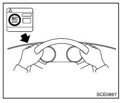
1. Open the lid of the air compressor and take out the speed restriction sticker, then put it in a location where the driver can see it while driving.
