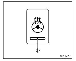
The heated steering wheel system is designed to operate only when the surface temperature of the steering wheel is below  $68^{\circ}F$  (20°C).
