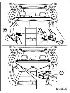
CARGO COVER (if so equipped for Hardtop models)
