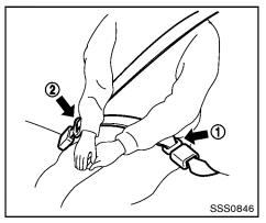
Rear center seat belt (Hardtop models) The rear center seat belt has a connector tongue (1) and a seat belt tongue (2). Both the connector tongue and the seat belt tongue must be securely latched for proper seat belt operation.
