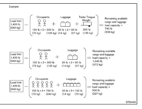
Steps for determining correct load limit
