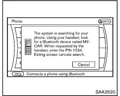
2. When a PIN code appears on the screen, operate the compatible Bluetooth  $^{\textcircled{B}}$  cellular phone to enter the PIN code.
