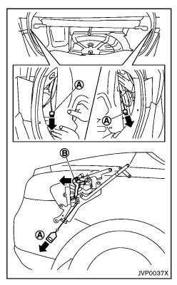
e. Pull back the left and right side trim in the trunk room, then pull the left and right
