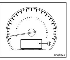
The dot matrix liquid crystal display ① is located in the speedometer, and it displays, the key operation information and other warnings and information.
