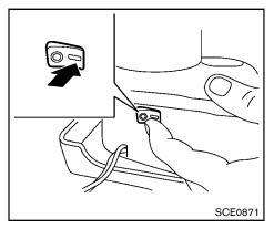
6. Push the ignition switch to the "ACC" position. Then turn the compressor switch to the ON (-) position and inflate the tire up to the pressure that is specified on the tire and loading information label affixed to the driver's side center pillar if possible, or to the minimum of 180 kPa (26 psi). Turn the air compressor off briefly in order to check the tire pressure with the pressure gauge.
