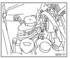
Check the fluid level in the reservoir.
