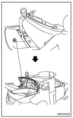
b. Lift the rear side of the soft top (A) until it is out of the storage area, then open the
