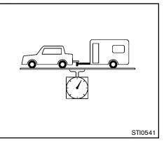
The GCWR equals the combined weight of the towing vehicle (including passengers and cargo) plus the total trailer load. Towing loads greater than these or using improper towing equipment could adversely affect vehicle handling, braking and performance.
