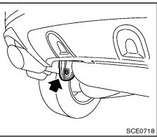
Tie down and recovery hook VEHICLE RECOVERY (freeing a stuck vehicle)
