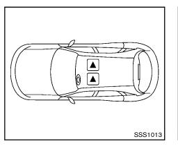
The illustration shows the seating positions equipped with head restraints. The head restraints are adjustable.
