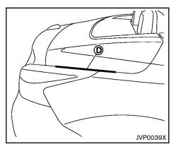
h. With two people, manually lift the storage lid by hand on the left and right side of the vehicle at lid edge D.
