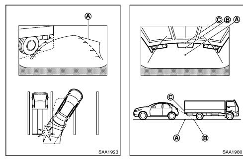
Backing up near a projecting object The predicted course lines (A) do not touch the object in the display. However, the vehicle may hit the object if it projects over the actual backing up course.
