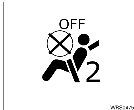
Front passenger air bag and status light
