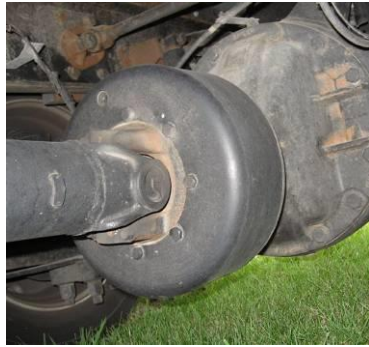
Example of driveline type and wheel type parking brakes
