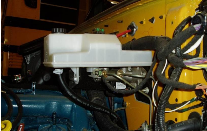
This is the firewall mounted master cylinder.
