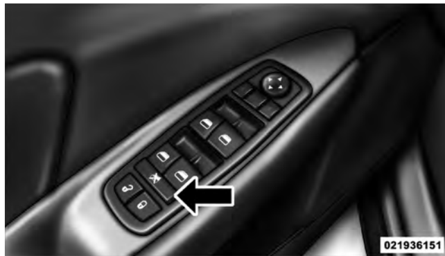
Window Lockout Switch
