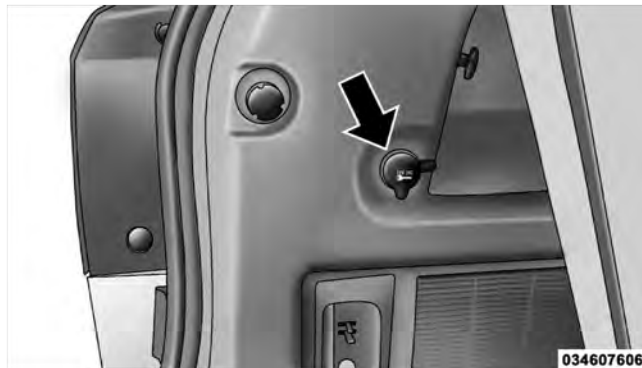
Rear Cargo Area Power Outlet
