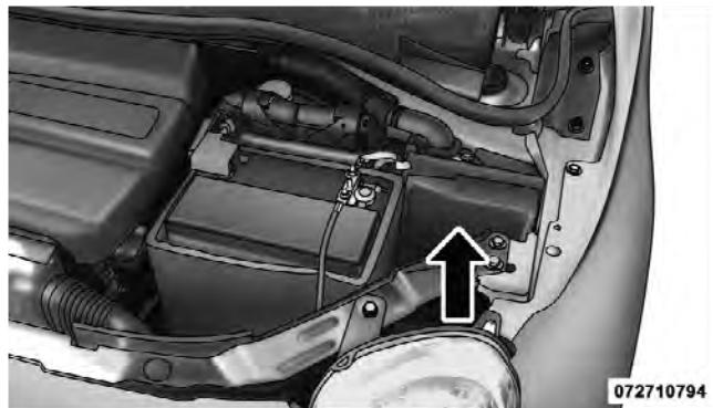
Front Distribution Unit
