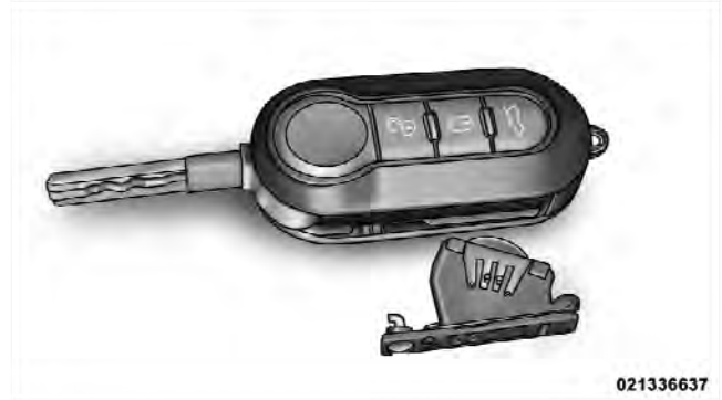
Battery Case Removed
