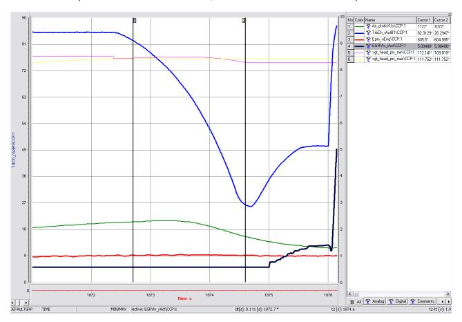
In the example above, at 1871 seconds, the EGR valve is commanded closed, after 3 seconds with EGR off and turbocharger at 85% position, the turbocharger is opened up to. 25% position. The 25% position is held for up to 10 seconds. If desired separation of 2kpa at sea level is achieved, the monitor aborts and the test is considered a pass. If desired separation isn't achieved, the monitor remains at 25% position for 10 seconds, and then the test is completed and failed.
