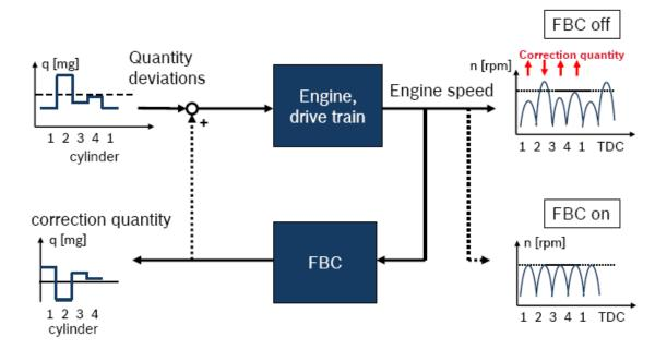
FBC operates in closed-loop control in an engine speed range of 500-1150 rpm, and a commanded injection quantity of 3.5-50 mg/stroke. The maximum allowed correction in fuel quantity for an individual cylinder is given by the following table.
