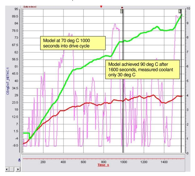
Warmup at -7 deg C on Unified Drive Cycle, DTC set when modeled temp reaches 90 deg C. Measured coolant temperature was only at 30 deg C.
