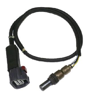
The NOx sensor control module is mounted to the vehicle frame under the body. It is used to control the combination tailpipe NOx and O2 sensor mounted in the diesel aftertreatment exhaust system downstream of the SCR and DPF. It communicates to the ECM via CAN to report NOx and O2 concentrations as well as sensor/controller errors.
