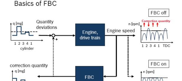
FBC operates in closed-loop control in an engine speed range of 500-1150 RPM, and a commanded injection quantity of 3.5-50 mg/stroke. The maximum allowed correction in fuel quantity for an individual cylinder is given by the following table.
