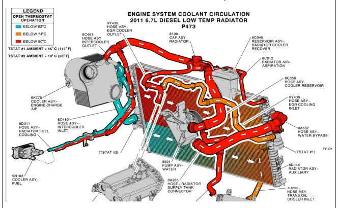
The dynamic check to detect a stuck ECT2 sensor is identical in function to the dynamic check used for the primary coolant loop. A minimum rise is expected over a calibratable amount of time,
