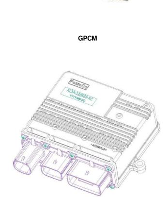
The GPCM is connected to the ECU via Diesel high speed CAN. All data and diagnostics pass over this non-public communication bus. The standard operating voltages for the GPCM are 6.5 volts to 16 volts. Limited operation between 5.5v and 6.5v on the lower range and no operation below 5.5v. Glow function is disabled below 6.5v and above 16.5v.
