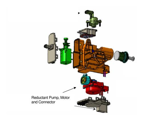
Reductant Pump Motor speed is controlled by a PWM driver in the engine ECU. Increasing the duty cycle of the PWM increases the Pump Motor speed. PWM duty cycles between 87 and 95 are reserved for diagnostics.
