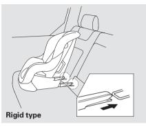
4. Place the child seat on the vehicle seat, then attach the seat to the lower anchors according to the child seat maker's instructions.
