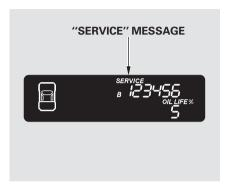
When the remaining engine oil life is 5 to 1 percent, you will see a "SERVICE" message along with the same maintenance item code(s), every time you turn the ignition switch to the ON (II) position.
