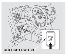
To turn off the lights, push the light switch again, or close the tailgate and the In-Bed Trunk.
