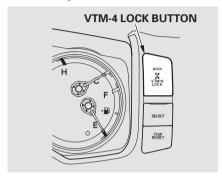
Your vehicle is equipped with a Variable Torque Management<sup>®</sup> 4-wheel-drive system (VTM-4<sup>®</sup>) that distributes engine torque to the appropriate drive axle depending on the available traction conditions. The system is completely automatic, always active, and does not require any driver interaction.
