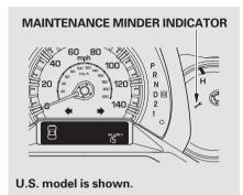
If the remaining engine oil life is 15 to 6 percent, you will see the engine oil life indicator every time you turn the ignition switch to the ON (II) position. The Maintenance Minder indicator will also come on, and the maintenance item code (s) for other scheduled maintenance items needing service will be displayed near the "OIL LIFE" message.
