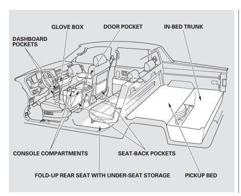
The pickup bed on your vehicle allows you to carry heavy and large cargo. You can also store items in the In-Bed Trunk and on a roof-rack (if equipped).
