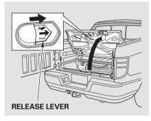
As a safety feature, your vehicle has a release lever on the latch of the In-Bed Trunk lid so it can be opened from the inside. To open the In-Bed Trunk, push the release lever in the direction of the arrow.
