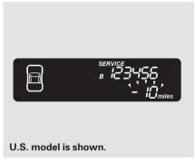
If you do not perform the indicated maintenance, negative distance traveled is displayed and begins to blink after the vehicle has been driven 10 miles (10 km) or more.
