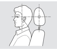
Adjust the driver's head restraint so the center of the back of your head rests against the center of the restraint.
