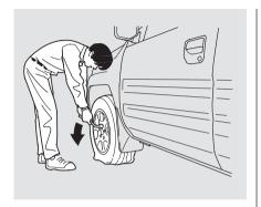
8. Loosen each wheel nut 1/2 turn with the wheel nut wrench.
