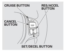
Push in the CRUISE button on the steering wheel. The CRUISE MAIN indicator on the instrument panel comes on.
