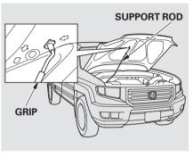
3. Holding the grip, pull the support rod out of its clip. Insert the end into the designated hole in the hood marked by an arrow.
