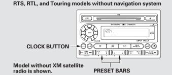
On models without navigation system If your vehicle's battery is disconnected or goes dead, you may need to set the clock.
