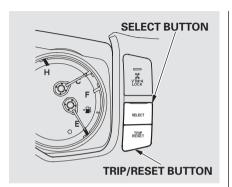
With the ignition switch in the ON (II) position, the information display changes as shown on the next page each time you press the SELECT button or TRIP/RESET button.
