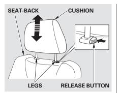
Adjusting the Head Restraint
