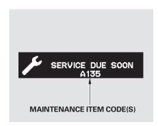
When the remaining engine oil life is 15 percent or less, the display shows a "SERVICE DUE SOON" message along with the maintenance item code(s) for other scheduled maintenance items needing service.
