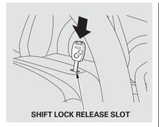
6. Remove the key from the shift lock release slot, then reinstall the cover. Make sure the notch on the cover is on the instrument panel side. Insert the key into the ignition switch, press the brake pedal, and restart the engine.
