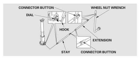
11.Attach the stay to the extension, then attach the wheel nut wrench to the end of the extension.
