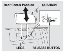
When a passenger is seated in the rear center seating position, make sure the center head restraint is properly positioned.
