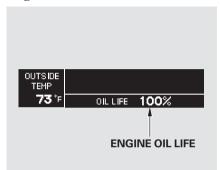
This shows the remaining life of the engine oil. It shows 100% after the engine oil is replaced and the display is reset. The engine oil life is calculated based on engine operating conditions and accumulated engine revolutions. For more information, see page 315.
