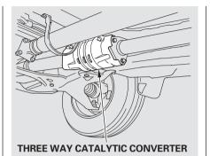
The defective three way catalytic converters contribute to air pollution, and can impair your engine's performance. Follow these guidelines to protect your vehicle's three way catalytic converters.
