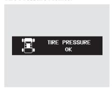
To select the tire pressure monitor, press the INFO button several times with the ignition switch in the ON (II) position.
