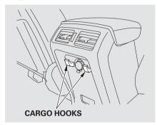
There are two cargo hooks for plastic grocery bags at the back of the center console. They are designed to hold light items. Heavy objects may damage the hooks.
