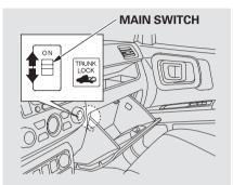
To protect items in the In-Bed Trunk, you can disable its release button by turning off the main switch in the glove box and locking the glove box with the master key.
