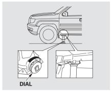
10. Turn the dial at the bottom of the jack clockwise until the top of the jack contacts the jacking point.
