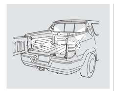
Your vehicle has bed lights in the pickup bed: a light on each front upper and rear bottom side. With the shift lever in the Park position, the bed lights come on when you push the bed light switch on the dashboard, swing open the tailgate, or open the In-Bed Trunk. The indicator on the instrument panel also comes on to remind you that the bed lights are on.
