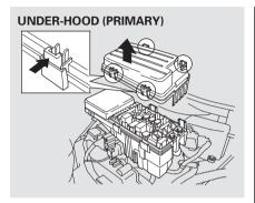
The primary under-hood fuse box is on the passenger's side. The secondary fuse box is next to the brake fluid reservoir. To open them, push the tabs as shown.
