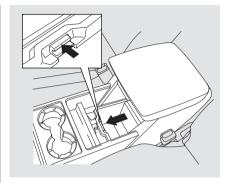
To open the rear of the compartment, push the button at the end of the tray, then slide the tray forward. To close, slide the tray back in place.
