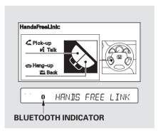
A notification that there is an incoming call, or HFL is in use, will appear on the navigation screen when the audio system is on.
