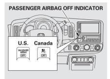
This indicator alerts you that the passenger's front airbag has been shut off because weight sensors detect about 65 lbs (29 kg) or less (the weight of an infant or small child) on the front passenger's seat. It does *not mean* there is a problem with the airbag.
