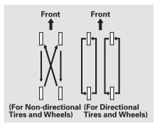
To help increase tire life and distribute wear more evenly, rotate the tires according to the maintenance messages displayed on the information display or multi-information display (depending on models). Move the tires to the positions shown in the diagram each time they are rotated. If you purchase directional tires, rotate only front-to-back.
