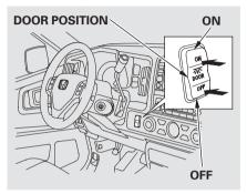
When the interior light control switch is in the ON position:
