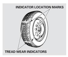
Your tires have wear indicators molded into the tread. When the tread wears down, you will see a 1/2 inch (12.7 mm) wide band across the tread. This shows there is less than 1/16 inch (1.6 mm) of tread left on the tire.
