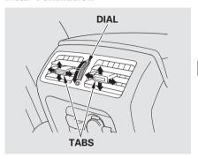
You can adjust the direction of the air coming from the rear vents in the back of the center console by moving the tab in the center of each vent up-and-down and side-to-side.
