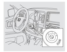
The ignition switch has four positions: LOCK (0), ACCESSORY (I), ON (II), and START (III).
