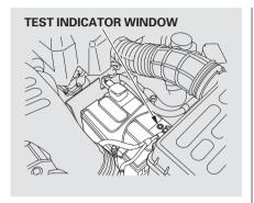
Check the condition of the battery monthly by looking at the test indicator window. The label on the battery explains the test indicator's colors. Check the terminals for corrosion (a white or yellowish powder). To remove it, cover the terminals with a solution of baking soda and water. It will bubble up and turn brown. When this stops, wash it off with plain water. Dry off the battery with a cloth or paper towel. Coat the terminals with grease to help prevent future corrosion.
