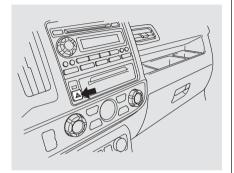
Push the button to turn on the hazard warning lights (four-way flashers). This causes all four outside turn signals and both turn indicators in the instrument panel to flash. Use the hazard warning lights if you need to park in a dangerous area near heavy traffic, or if your vehicle is disabled.
