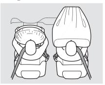
Your vehicle has a supplemental restraint system (SRS) with front airbags to help protect the heads and chests of the driver and a front seat passenger during a moderate to severe frontal collision (see page 25 for more information on how your front airbags work).
