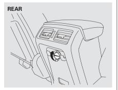
These sockets are intended to supply power for 12 volt DC accessories that are rated 120 watts or less (10 amps).
