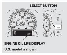
To see the current engine oil life, turn the ignition switch to the ON (II) position, and press the SELECT button repeatedly until the engine oil life display appears (see page 78).
