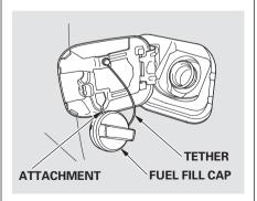
3. Remove the fuel fill cap slowly. You may hear a hissing sound as pressure inside the tank escapes. The fuel fill cap is attached to the fuel filler with a tether. Insert the attachment on the fuel fill cap into the slit on the fuel fill door.
