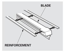
5. Examine the new wiper blades. If they have no plastic or metal reinforcement along the back edge, remove the metal reinforcement strips from the old wiper blade, and install them in the slots along the edge of the new blade.
