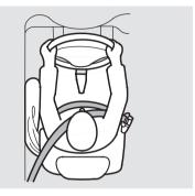
If you ever have a moderate to severe side impact, sensors will detect rapid acceleration and signal the control unit to instantly inflate either the driver's or the passenger's side airbag.
