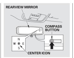
The direction and center position icons come on when you turn the ignition switch to the ON (II) position. The system then begins to check the vehicle direction and illuminates the appropriate icon(s).
