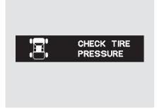
Each tire has its own pressure sensor. If the air pressure of a tire becomes significantly low, the sensor in that tire immediately sends a signal that causes the low tire pressure/TPMS indicator in the instrument panel to come on. If this happens, you will see which tire is losing pressure on the multi-information display along with a "CHECK TIRE PRESSURE" message.
