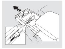
To open the front of the compartment, squeeze the knob, and push it forward while sliding the beverage holder. To close, squeeze the knob and pull the compartment backward until the beverage holder latches.
