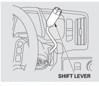
To shift from Park to any position, press firmly on the brake pedal, and pull the shift lever toward you. You cannot shift out of Park when the ignition switch is in the LOCK (0) or ACCESSORY (I) position.
