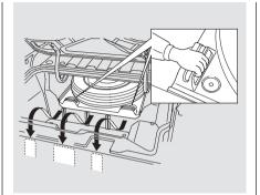
5. Pull out the tire tray with the handle, and hook the rear of the tire tray to the guides on the back edge of the In-Bed Trunk.
