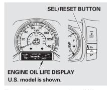
To see the current engine oil life, turn the ignition switch to the ON (II) position, and push and release the SEL/RESET button on the dashboard repeatedly, until the engine oil life is displayed (see page 83).
