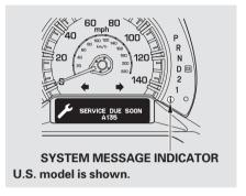
The system message indicator on the instrument panel will also come on, and a beeper will sound. To cancel the system message, press and release the INFO  $(\blacktriangle/\blacktriangledown)$  button on the dashboard. At this time, the system message indicator will also be turned off. Then the display will change to the engine oil life display.
