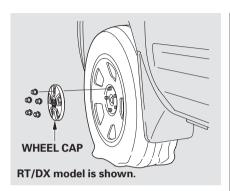
14.Remove the wheel nuts and the wheel cap (on RT and DX models) then remove the flat tire. Handle the wheel nuts carefully; they may be hot from driving. Place the flat tire on the ground with the outside surface facing up.
