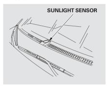
The climate control system has two sensors. A sunlight sensor is in the top of the dashboard, and a temperature sensor is under the steering column. Do not cover the sensors or spill any liquid on them.
