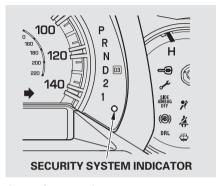
Once the security system sets, opening any door (without using the key or the remote transmitter), the hood, or the In-Bed Trunk, will cause the alarm to activate. It also activates if the radio and navigation components are removed from the dashboard or the wiring is cut.
