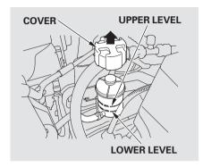
Remove the cover, then check the level on the side of the reservoir when the engine is cold.
