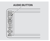
To adjust the sound, push the AUDIO button, then enter the sound grid by touching the SOUND icon on the display.
