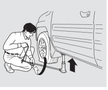
13. Turn the jack dial (wheel nut wrench) clockwise as shown to raise the vehicle until the flat tire is off the ground.
