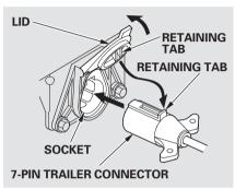
The 7-pin trailer connector is needed for the trailer lights. To connect the connector:
