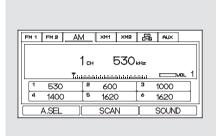
On models with navigation system In addition to the knobs, buttons, and bars on the radio control panel, you can operate some of the radio controls on the navigation system screen. While you are listening to the radio, you can change to another band by pressing the AUDIO button next to the navigation system screen, and then touching the desired band icon (FM1, FM2, or AM).
