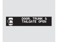
When the In-Bed Trunk, tailgate, and one or more doors are not tightly closed, the "DOOR, TRUNK & TAILGATE OPEN" message will come on.
