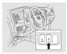
This switch is above the parking brake release handle. To turn the VSA system on and off, press and hold it until you hear a beep.
