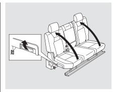
To fold a rear seat cushion, pull up the lever on the outside of the cushion. The seat cushion pops up, and the seat legs store underneath it. Push the cushion firmly against the seat-back to lock it in place.
