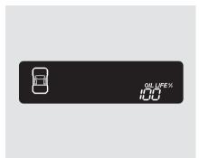
4. Press the TRIP/RESET button for another 5 seconds. The maintenance item code(s) will disappear, and the engine oil life will reset to "100." On models with navigation system
