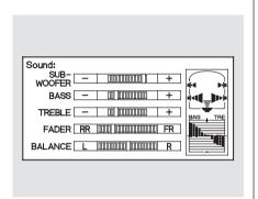
**Treble/Bass** — To adjust the treble and bass, touch + or — on each side of the treble or bass adjustment bar. The adjustment bar shows you the current setting.
