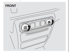
There are three accessory power sockets in your vehicle. Two accessory power sockets are above the center pocket on the dashboard, and another is on the back of the center console.
