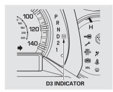
When D3 is on, the transmission selects only the first three gears. Use D3 for engine braking when going down a steep hill.
