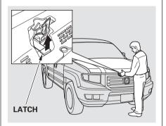
2. Put your fingers under the front edge of the hood. The hood latch handle is above the "H" logo. Pull this handle until it releases the hood, then lift the hood.
