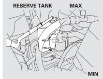
Look at the coolant level in the radiator reserve tank. Make sure it is between the MAX and MIN lines. If it is below the MIN line, see **Adding Engine Coolant** on page 331 for information on adding the proper coolant.
