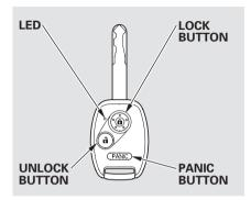
**LOCK** — Press this button once to lock all doors and the In-Bed Trunk. Some exterior and interior lights will flash once.
