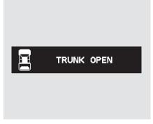
When the In-Bed Trunk is not tightly closed, the "TRUNK OPEN" message will come on.
