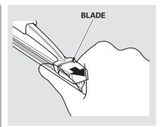
4. Remove the blade from its holder by grabbing the tabbed end of the blade. Pull up firmly until the tabs come out of the holder.
