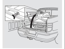
To close the In-Bed Trunk, lower the lid, then press down on the back edge.
