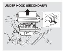
Checking and Replacing Fuses If something electrical in your vehicle stops working, check for a blown fuse first. Determine from the chart on pages 383 and 384, or the diagram on the fuse box lid, which fuse or fuses control that device. Check those fuses first, but check all the fuses before deciding that a blown fuse is the cause. Replace any blown fuses, and check if the device works.
