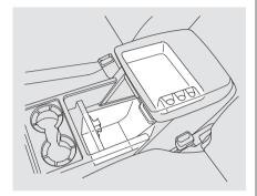
Your vehicle has a multi-function center console. It includes beverage holders, storage compartments, an armrest, a coin holder, and a storage tray.
