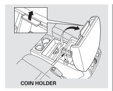
You can put small items in the upper console compartment. To use it, pull up on the lever and lift up the armrest.
