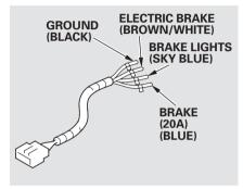
The trailer jumper harness is used to install the controller for the electric trailer brakes. For more information, see *Trailer Brakes* on page 300.
