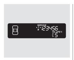
3. Press the TRIP/RESET button for about 10 seconds. The engine oil life and the maintenance item code(s) will blink.
