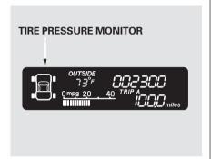
The appropriate tire indicator will come on along with the low tire pressure indicator if a tire is significantly underinflated or has suddenly lost pressure. See **Low Tire Pressure Indicator** for what to do if this indicator comes on.
