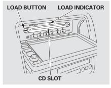
1. Press and hold the LOAD button next to the CD slot until the load indicator above the slot turns from amber to green.
