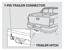
Your vehicle has a class 3 trailer hitch as standard equipment.
