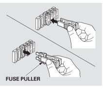
4. Check the smaller fuses in the under-hood fuse boxes and all the fuses in the interior fuse box by pulling out each one with the fuse puller provided in the primary under-hood fuse box.
