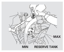
If the coolant level in the reserve tank is at or below the MIN line, add coolant to bring it up to the MAX line. Inspect the cooling system for leaks.
