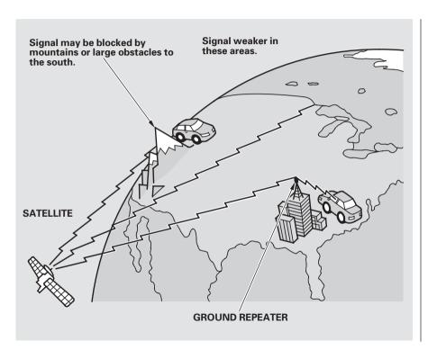
The XM satellites are in orbit over the equator; therefore, objects south of the vehicle may cause satellite reception interruptions. To help compensate for this, ground-based repeaters are placed in major metropolitan areas.
