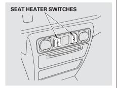
Push the top of the switch, HI, to rapidly heat up the seat. After the seat reaches a comfortable temperature, select LO by pushing the bottom of the switch. This will keep the seat warm.
