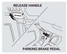
To apply the parking brake, push the pedal down with your foot. To release it, pull the release handle fully. The parking brake indicator on the instrument panel should go out when the parking brake is fully released (see page 65).
