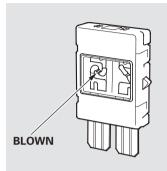
3. Check each of the large fuses in the primary under-hood fuse box by looking through the side window at the wire inside. Removing these fuses requires a Phillips-head screwdriver.
