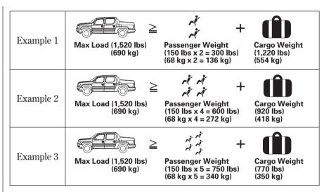
In addition, the total weight of the vehicle, all occupants, accessories, cargo, and trailer tongue load must not exceed the Gross Vehicle Weight Rating (GVWR) or the Gross Axle Weight Rating
