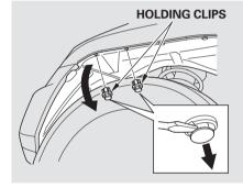
2. Use a flat-tip screwdriver to remove the two holding clips from the inner fender, and pull the inner fender cover back.
