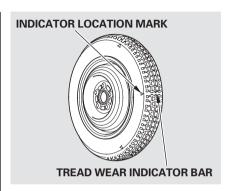
Replace the tire when you can see the tread wear indicator bars. The replacement tire should be the same size and design, mounted on the same wheel. The spare tire is not designed to be mounted on a regular wheel, and the spare wheel is not designed for mounting a regular tire.
