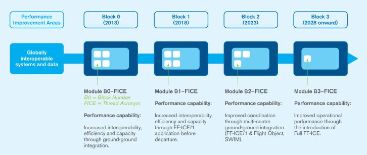
Fig. 4: A Module Thread is associated with a specific Performance Improvement Area. Note that the Modules in each consecutive Block feature the same Thread Acronym (FICE), indicating that they are elements of the same Operational Improvement process.
