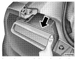
7. Push the electrical connector locking tab to the side.
