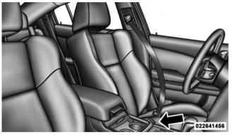
**Inserting Latch Plate Into Buckle**
