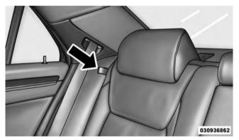
**Rear Seatback Loop** After releasing the seatback, it can be folded forward.
