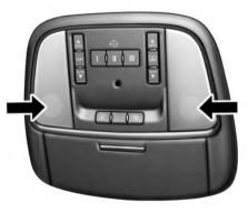
To turn the lights off, press the switch a second time. The lights also turn on when a door is opened. The lights will also turn on when the UNLOCK button on the RKE is pressed.
