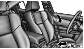
Pulling Out The Lap/Shoulder Belt Latch Plate
