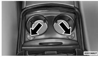
Heated And Cooled Cupholder Switches
