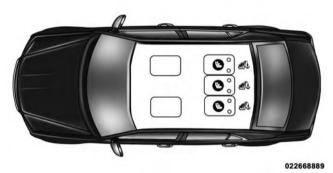
Lower Anchorage Symbol 2 anchorages per seating position
