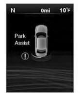
The vehicle is close to the obstacle when the warning display shows one flashing arc and sounds a continuous tone. The following chart shows the warning alert operation when the system is detecting an obstacle:
