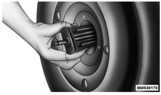
**Removing Wheel Spacer**
