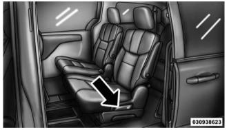
Seatback Recliner Lever, Seat Tumble, And Head Restraint Fold Lever The non-adjustable head restraint and seatback will fold automatically during the seat tumble. No additional actuation is necessary.
