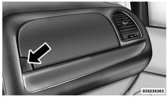
**Upper Compartment** To close the compartment door, push downward on the door's surface to latch the door closed.
