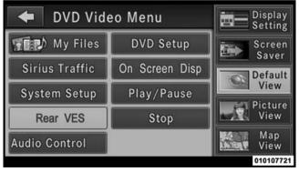
3. Touch the 1 soft-key and then touch either AUX 1 or AUX 2 in the VES column (depending which AUX input is used). To exit press the back arrow soft-key at the top of the screen.
