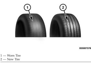
These indicators are molded into the bottom of the tread grooves. They will appear as bands when the tread depth becomes 1/16 in (2 mm). When the tread is worn to the tread wear indicators, the tire should be replaced. Refer to replacement tires in this section for further information.
