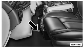
Winch Cover Assembly Plug (If Equipped) Spare Tire Tools
