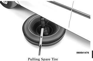
**NOTE:** If either front tire is flat it may be necessary to jack up the vehicle to remove the compact spare tire/ cover assembly from under the vehicle.
