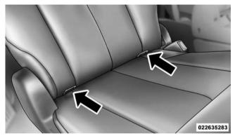
LATCH Anchorages (Second Row Anchorages Shown)
