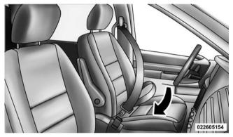
Inserting Latch Plate Into Buckle
