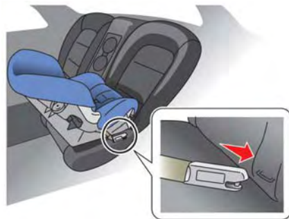
Rear-facing rigid-mounted — step 2
