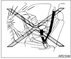
Bag System, never install a rear-facing child restraint in the front seat. An inflating front air bag could seriously injure or kill your child. See "Child restraints" earlier in this section for details.
