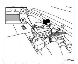
Check the fluid level in the reservoir. If the brake fluid is below the MIN line (B), the brake warning light will illuminate. Add brake fluid up to the MAX line(A). (See "RFCOMMENDED FUEL/LUBRICANTS AND CAPACITIES" in the " Technical and consumer information" section for the recommended type of brake fluid.)
