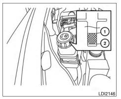
Check the fluid level in the reservoir.
