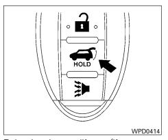
Releasing the rear liftgate (if so equipped)
