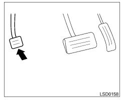
**To engage:** Firmly depress the parking brake.
