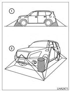
There are some areas where the system will not show objects. When in the front or rearview display, an object below the bumper or on the ground may not be viewed ①. When in the bird-eye view, a tall object near the seam of the camera viewing areas will not appear in the monitor ②.
