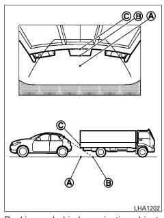
Backing up behind a projecting object The position © is shown farther than the position ® in the display. However, the position © is actually at the same distance as the position A. The vehicle may hit the object when backing up to the position A if the object projects over the actual backing up course.
