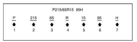
H: Tire speed rating. You should not drive the vehicle faster than the tire speed rating.
