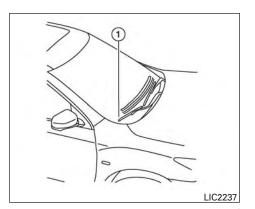
Be sure you do not put anything on top of the autolight sensor located in the top side (1) of the instrument panel. The autolight sensor controls the autolight: if it is covered, the autolight sensor reacts as if it is dark out and the headlights will illuminate. If this occurs while parked with the engine off and the ignition switch placed in the ON position, your vehicle's battery could become discharged.
