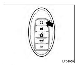
The **Q** button will be on the NISSAN Intelligent Key® if the vehicle has remote engine start. This feature allows the engine to start from outside the vehicle.
