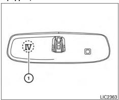
The Type B system can be identified by the IV (1) on the back of the mirror. Move the mirror to see if the IV is present. If the IV is on the mirror, use the procedure in this section to program the HomeLink® Universal Transceiver . Otherwise. use the procedure in "HomeLink® universal transceiver (Type A) (if so equipped)".
