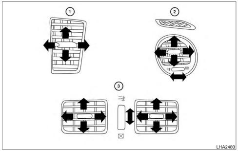
Adjust air flow direction for the driver's and passenger's side vents ①, center vents ②, and rear vents 3 by moving the vent slide and/or vent assemblies.
