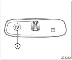
The Type A system does not have an IV (1) on the back of the mirror. Move the mirror to see if the IV is present. If the IV is not on the mirror, use the procedure in this section to program the HomeLink® Universal Transceiver, If the IV is on the mirror, use the procedure in "HomeLink® universal transceiver (Type B) (if so equipped)".
