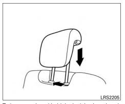
To lower, push and hold the lock knob and push the headrest down.
