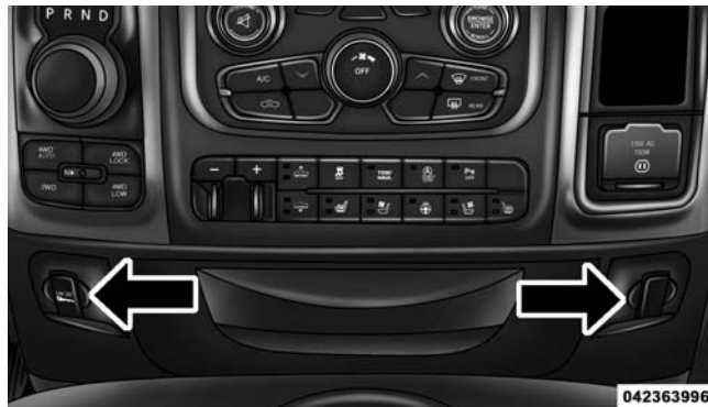
Power Outlets — Center Stack
