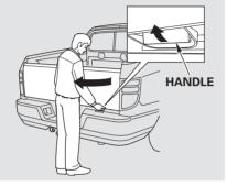
To swing open the tailgate, first make sure it is fully closed, then pull up the right lower handle, and swing the tailgate to the left. To close, swing the tailgate back, and push it firmly until it is latched.
