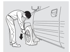
8. Loosen each wheel nut 1/2 turn with the wheel nut wrench.
