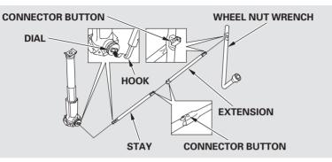
11.Attach the stay to the extension, then attach the wheel nut wrench to the end of the extension.
