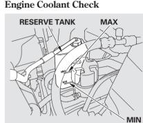
Look at the coolant level in the radiator reserve tank. Make sure it is between the MAX and MIN lines. If it is below the MIN line, see **Adding Engine Coolant** on page 327 information on adding the proper proper coolant.
