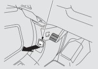
1. Park the vehicle, and set the parking brake. Pull the hood release handle under the lower left corner of the dashboard. The hood will pop up slightly.
