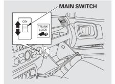
To protect items in the In-Bed Trunk, you can disable its release button by turning off the main switch in the glove box and locking the glove box with the master key.
