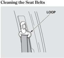
If your seat belts get dirty, use a soft brush with a mixture of mild soap and warm water to clean them. Do not use bleach, dye, or cleaning solvents. Let the belts air-dry before you use the vehicle. Dirt build-up in the loops of the seat belt anchors can cause the belts to retract slowly. Wipe the insides of the loops with a clean cloth dampened in mild soap and warm water or isopropyl alcohol.
