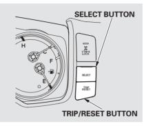
With the ignition switch in the ON (II) position, the information display changes as shown on the next page each time you press the SELECT button or TRIP/RESET button.
