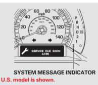
The system message indicator on the instrument panel will also come on, and a beeper will sound. To cancel the system message, press and release the INFO ( $\checkmark/\checkmark$ ) button on the dashboard. At this time, the system message indicator will also be turned off. Then the display will change to the engine oil life display.
