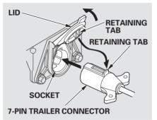
The 7-pin trailer connector is needed for the trailer lights. To connect the connector:
