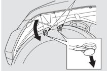
2. Use a flat-tip screwdriver to remove the two holding clips from the inner fender, and pull the inner fender cover back.
