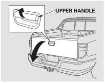
To drop open the tailgate, pull up the upper handle, then pull down the tailgate. To close the tailgate, push firmly up until it latches.
