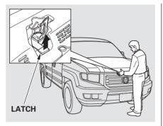
2. Put your fingers under the front edge of the hood. The hood latch handle is above the "H" logo. Pull this handle until it releases the hood, then lift the hood.
