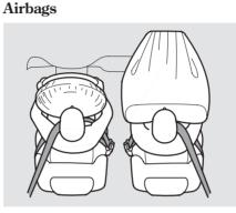
Your vehicle has a supplemental restraint system (SRS) with front airbags to help protect the heads and chests of the driver and a front seat passenger during a moderate to severe frontal collision (see page 25 for more information on how your front airbags work).
