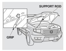
3. Holding the grip, pull the support rod out of its clip. Insert the end into the designated hole in the hood marked by an arrow.
