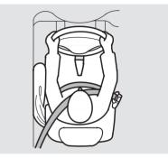
If you ever have a moderate to severe side impact, sensors will detect rapid acceleration and signal the control unit to instantly inflate either the driver's or the passenger's side airbag. 1
