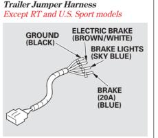
The trailer jumper harness is used to install the controller for the electric trailer brakes. For more information, see *Trailer Brakes* on page 296.
