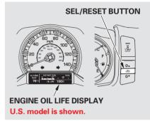
To see the current engine oil life, turn the ignition switch to the ON (II) position, and push and release the SEL/RESET button on the dashboard repeatedly, until the engine oil life is displayed (see page 83).
