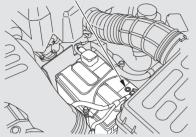
Check the condition of the battery monthly by looking at the test indicator window. The label on the battery explains the test indicator's colors. Check the terminals for corrosion (a white or yellowish powder). To remove it, cover the terminals with a solution of baking soda and water. It will bubble up and turn brown. When this stops, wash it off with plain water. Dry off the battery with a cloth or paper towel. Coat the terminals with grease to help prevent future corrosion.
