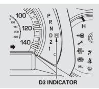
When D3 is on, the transmission selects only the first three gears. Use D3 for engine braking when going down a steep hill. When towing a trailer on level roads under normal driving conditions, do not use D3. This will increase the automatic transmission fluid temperature and may cause overheating.
