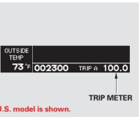
This meter shows the number of miles (U.S.) or kilometers (Canada) driven since you last reset it. There are two trip meters: Trip A and Trip B. Each trip meter works independently, so you can keep track of two different distances.
