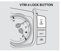
Your vehicle is equipped with a Variable Torque Management<sup>®</sup> 4-wheel-drive system (VTM-4<sup>®</sup>) that distributes engine torque to the appropriate drive axle depending on the available traction conditions. The system is completely automatic, always active, and does not require any driver interaction.
