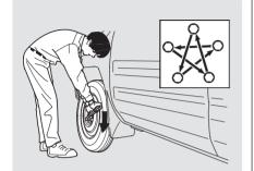
18. Tighten the wheel nuts securely in the same crisscross pattern. Have the wheel nut torque checked at the nearest automotive service facility.
