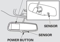
Whenever you shift to reverse (R) with the ignition switch in the ON (II) position, the rear view appears on a display in the rearview mirror.
