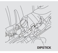
2. Remove the dipstick (yellow loop) from the transmission, and wipe it with a clean cloth.
