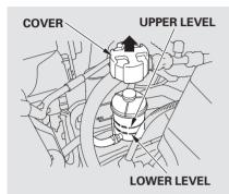
Remove the cover, then check the level on the side of the reservoir when the engine is cold. The fluid should be between the UPPER LEVEL and LOWER LEVEL. If not, add power steering fluid to the UPPER LEVEL mark, and put the cover back in place. Pour the fluid slowly and carefully so you do not spill any. Clean up any spill immediately; it could damage components in the engine compartment.
