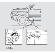
10. Turn the dial at the bottom of the jack clockwise until the top of the jack contacts the jacking point. Make sure the jacking point tab is resting in the jack notch.
