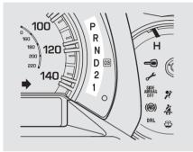
These indicators on the instrument panel show which position the shift lever is in. The "D" indicator comes on for a few seconds when you turn the ignition switch to the ON (II) position. If it flashes while driving (in any shift position), it indicates a possible problem in the transmission.
