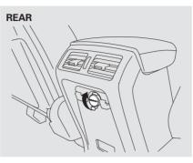
These sockets are intended to supply power for 12 volt DC accessories that are rated 120 watts or less (10 amps).
