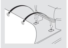
A non-Honda floor mat may not fit your vehicle properly. This could prevent the proper operation of the folding rear seats and the passenger's seat weight sensors. We recommend using genuine Honda floor mats. Do not put additional floor mats on top of the anchored mats.
