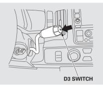
Press the D3 switch on the end of the shift lever to turn this mode on or off; the D3 indicator comes on whenever D3 is selected.
