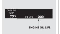
This shows the remaining life of the engine oil. It shows 100% after the engine oil is replaced and the display is reset. The engine oil life is calculated based on engine operating conditions and accumulated engine revolutions. For more information, see page 311.
