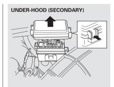
**Checking and Replacing Fuses** If something electrical in your vehicle stops working, check for a blown fuse first. Determine from the
