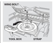
6. Unfasten the strap to remove the tool box, and unscrew the wing bolt.
