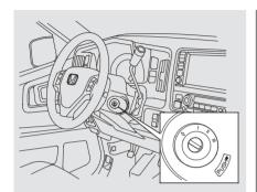
The ignition switch has four positions: LOCK (0), ACCESSORY (I), ON (II), and START (III). LOCK (0) – You can insert or remove the key only in this position. To turn the key, the shift lever must be in Park, and you must push the key in slightly.
