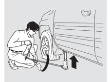
13.Turn the jack dial (wheel nut wrench) clockwise as shown to raise the vehicle until the flat tire is off the ground.
