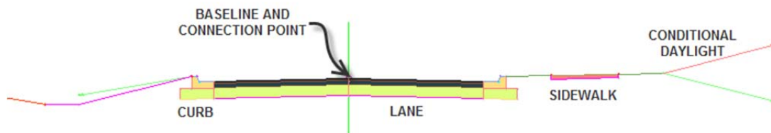
Figure 15: An assembly is made of up a combination of subassemblies such as sidewalks, curbs, and lanes.
