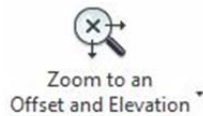
Figure 36: To keep views consistent when viewing corridor section results, use the Zoom to an Offset and Elevation option.
