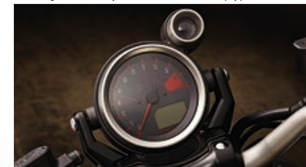
Handlebar-mounted meter includes tachometer and digital speedo plus an adjustable shift light.
