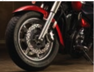
Dual 298-mm floating front discs.
