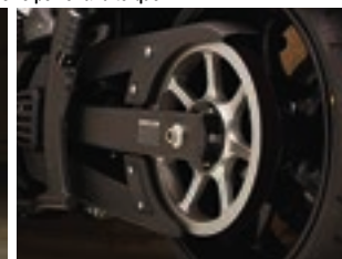
Clean, quiet low-maintenance belt drive.
