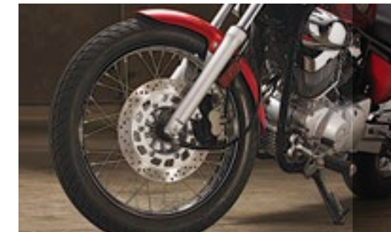
Spoked, chrome wheels fitted with a narrow front and wide 130-series rear tire.
