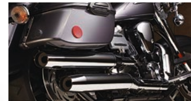
2-into-2 exhaust system features beefy, staggered, dual shotgun pipes.
