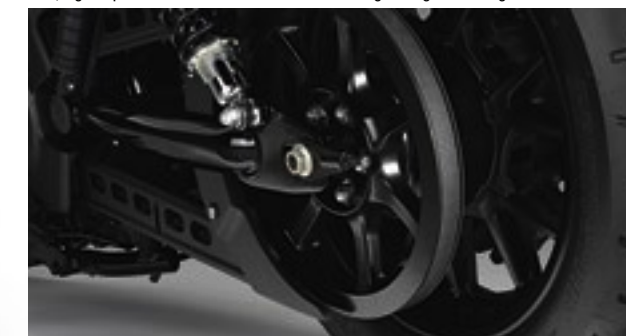
Clean, quiet belt drive system is extremely low-maintenance and simplifies customization.
