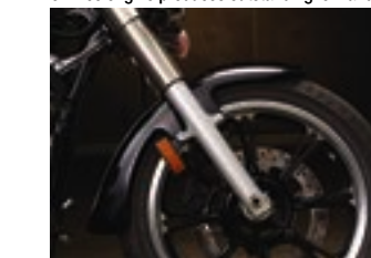
Lightweight 8-spoke cast aluminium wheels.
