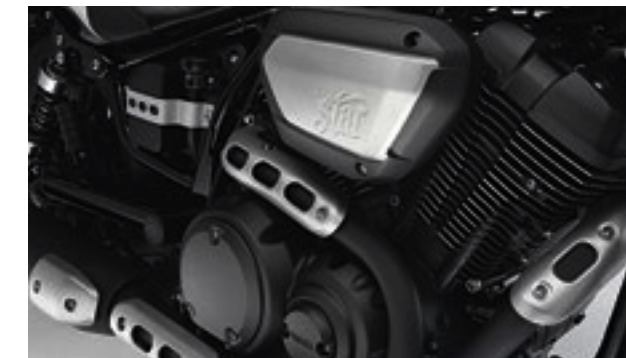
942 cc V-twin engine produces outstanding low and mid-range torque.
