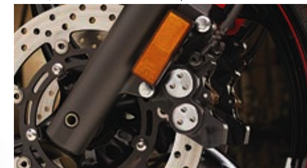
Dual 298-mm floating front discs are squeezed by ultra-rigid, 4-piston, monoblock calipers.
