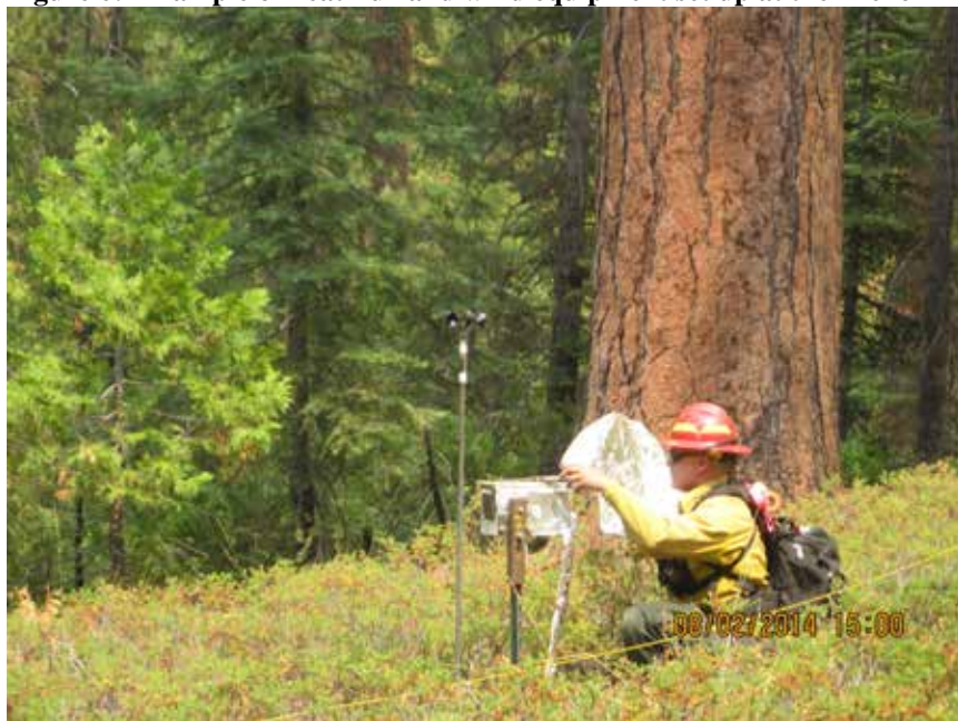
Figure 6: Example of heat flux and wind equipment set up at the French Fire in an open, mixed conifer area.
