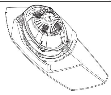
Step 6. Next you will attach the speaker, grille and mounting ring to the lid using the supplied screws.
