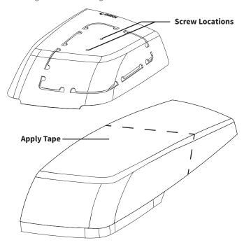
Step 3. Apply the template to the saddlebag lid and secure using (2) screws that came with the kit.
