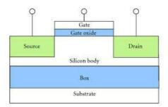
Figure 1: SOI MOSFET Structure
