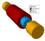
Figure 6: GAA MOSFET Structure
