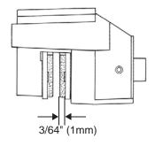
5. Inspect the brake disc spline and pad wear surface for excessive wear. Change pads when worn to 3/64" (1 mm).
