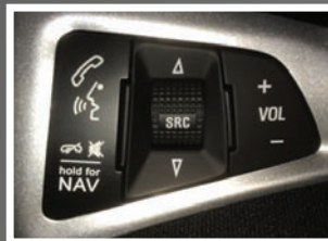
Replacement switch (hold for NAV)
