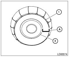
Use of tire chains may be prohibited according to location. Check the local laws before installing tire chains. When installing tire chains, make sure they are the proper size for the tires on your vehicle and are installed according to the chain manufacturer's suggestions. Use a tire chain that is designed to provide the specified space (A) between the installed tire chain (1) and where the tire meets the rim (2) as shown on the chart.
