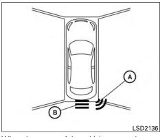
When the corner of the vehicle moves closer to an object, the corner sonar indicators (A) appears. When the center of the vehicle moves close to an object, the center sonar indicator (B) appears.
