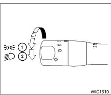
Type C (if so equipped) HEADLIGHT CONTROL SWITCH
