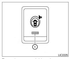
The warning systems switch is used to temporarily turn off the warning systems (Lane Departure Warning (LDW) and Blind Spot Warning (BSW) systems) that are activated using the settings menu in the vehicle information display.
