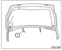
To fold down the driver's side of the rear seat, open the trunk and pull on the strap ①.
