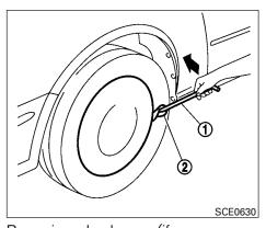
Removing wheel cover (if so equipped)
