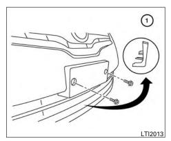
To mount the front license plate, attach the license plate bracket (1) to the plastic finisher at the location marks (small dimples) using the two 6 mm screws provided.
