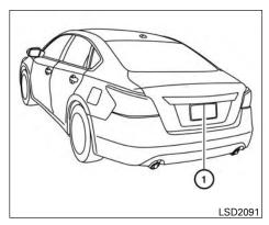
The BSW/LDW systems use the rear view monitor camera unit (1) with automatic washer and blower.
