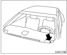
The sunload sensor, located on the top driver's side of the instrument panel, helps the system maintain a constant temperature. Do not put anything on or around this sensor.
