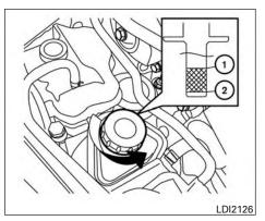
Check the fluid level in the reservoir.
