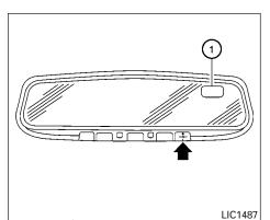
Press the -N- button for about 1 second when the ignition switch is placed in the ON position to toggle the compass display 1 on or off. The display will indicate the direction of the vehicle's heading.
