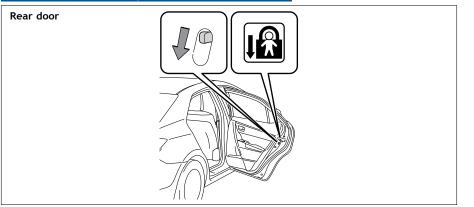
Pushing down the lever will allow the door to be opened only from the outside.
