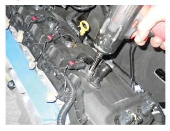
13. Remove the ignition coils and number them so they can be reinstalled in the position from which they were removed.
