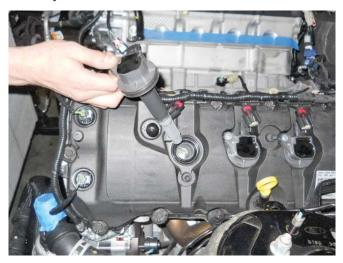
14. Using a 14 mm spark plug socket and a 6" extension, remove all eight (8) spark plugs.
