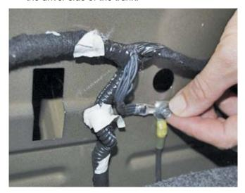
Plug the Intermediate harness into both the factory wiring harness and the fuel pump module.
