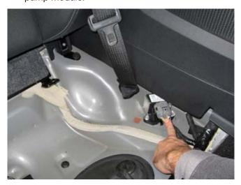
4. Remove the spare tire well cover and the emergency tire repair kit.
