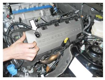
11. Disconnect the electrical connectors for each of the ignition coils.
