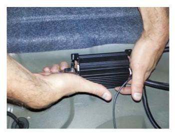
4. Attach the ground strap to the chassis ground of the driver side of the trunk.
