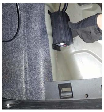
Using the 1/8" drill bit, drill the four (4) locations marked.
