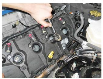
Unpack the eight (8) provided spark plugs (M-12405-M50), YOU MUST RE-GAP PLUGS TO 0.9 mm (.035") and verify that the plugs are not damaged.
