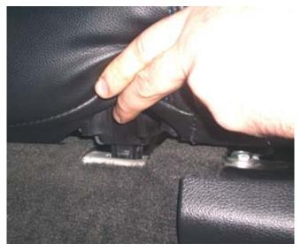
3. Disconnect the vehicle harness from the fuel pump module.
