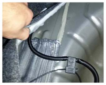
7. Connect the feed to the intermediate fuel pump harness connector. Make sure the harness is pointed out of the way of the rear seat cushion.
