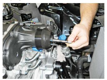
10. Re-install the FEAD belt on the supercharger by rotating the tensioner clockwise and routing the belt as shown in the routing below.
