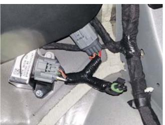
6. Run the 2-pin connector from the trunk well along the driver side panel to the fuel pump module.
