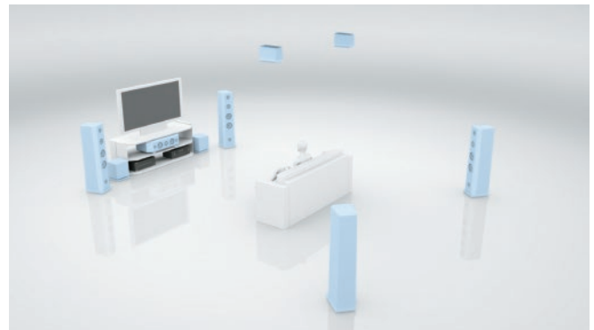
Speaker Layout Example of a Dolby Atmos Home Theater (5.2.2ch)
