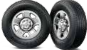
18-inch Steel, Argent Painted Finish Standard on 3500 Tradesman • Optional on 2500 Tradesman (WBN)
