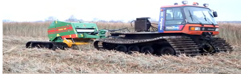
FIGURE 20. Modified Piston Bully harvesting reed ( Phragmites sp.) in Germany. Apparently, the unit converts hydraulics to run the PTO driven baler. Note the track-equipped baler and the supplemental radiator for additional cooling capacity of the hydraulic system.
