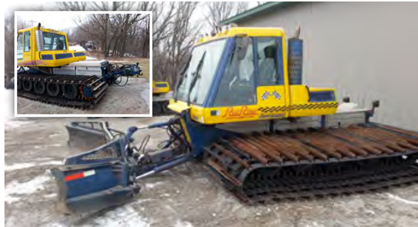
FIGURE 21. Bombardier trail groomer with front and rear hydraulics for powering implements.
