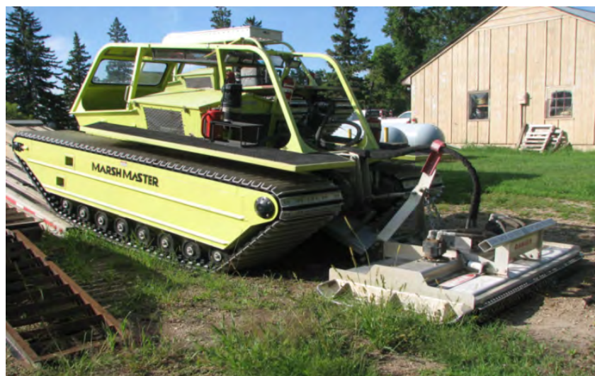
FIGURE 27. Marshmaster with rear mounted, hydraulically powered mower.
