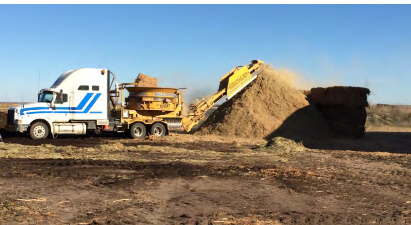
FIGURE 31. Industrial tub grinder processing cattails in Manitoba.
