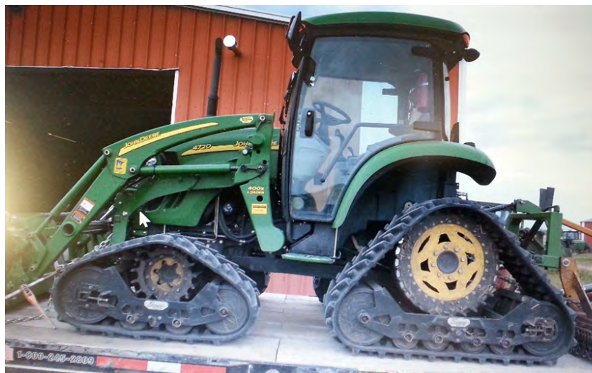
FIGURE 28. An example of a track-equipped tractor used by the Minnesota Department of Natural Resources for grassland and wetland prescribed burning. Such a unit could have a role in cattail harvesting.
