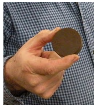
FIGURE 34. Torrefied cattail briquette ("hockey puck") made by Tim Hagen, Natural Resources Research Institute, U of MN, Duluth.
