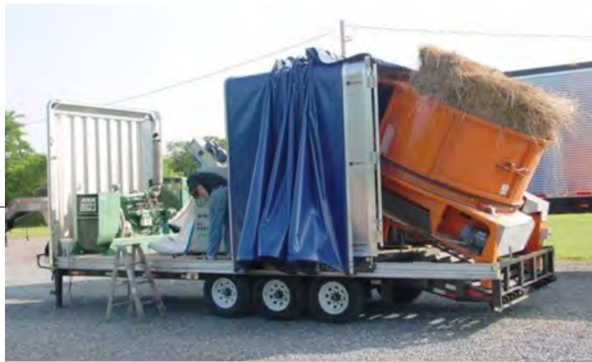
FIGURE 32. A mobile pelletizer made by Buskirk engineering. Note the self-contained tub-grinder.
