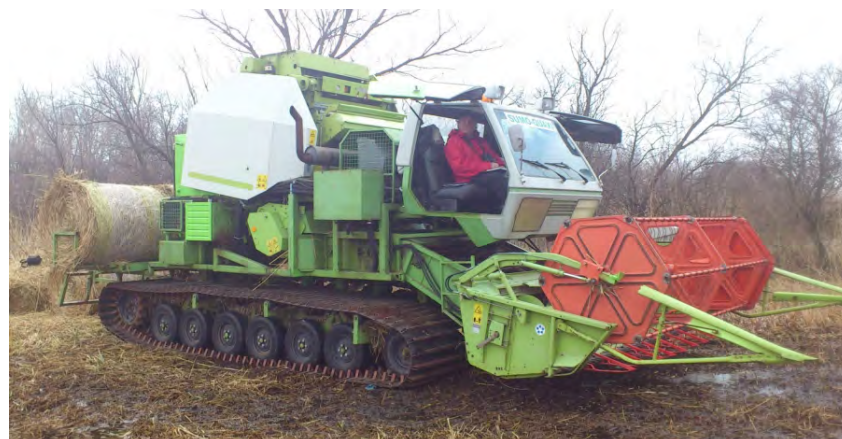
FIGURE 22. A single pass, swather/baler combination from Austria for harvesting reed. Made by Sumo Quaxi. http://duene-greifswald.de/doc/rrr2013/talks/Harvesting%20Techniques%20Beckmann%202013%20-%20Harvesting%20Technologies%20for%20reeds%20in%20Austria.pdf . Accessed 20 July 2016.
