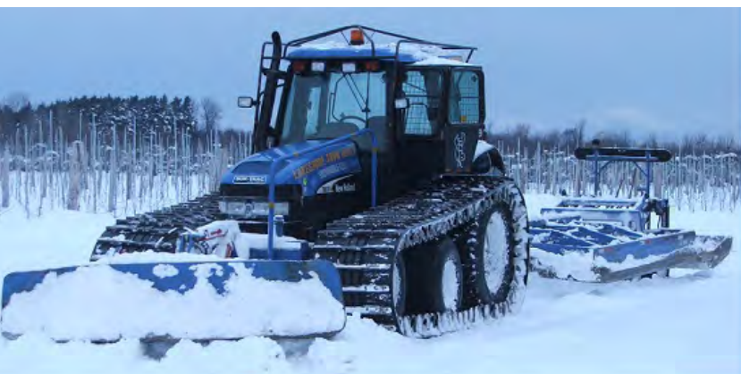
FIGURE 25. Conventional tractor adapted for trail grooming from New York.
