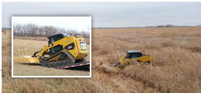
FIGURE 26. Front-mounted, hydraulically driven mower attached to skid-steer. Used to mow checker - board pattern at Parnell Flood Control Impoundment (Figure 12).
