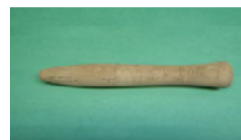
19. Bullet Reverse Payne, Up-Lock 6 1/2' .312 Hole, R44 Seat
