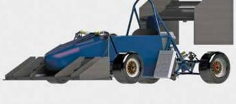
This year's car UTR-22, was built around simplicity and reliability while also taking on some new features. Utilizing tire consortium data as a starting point, UTR-22 features a rigid tubular chassis, CBR600 F4i, and Ohlins shocks backed up with extensive durability testing. Serviceability and weight reduction were also considered with every component designed. With a large amount of time dedicated to testing and refining we hope to have an all-around reliable and fine-tuned car for competition.
