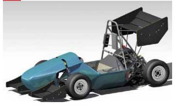
Poly eRacing is an all-electric formula SAE team which started from nothing in 2009. Our first prototype, unveiled at the summer of 2012, never competed in a dynamic event. The 2016 prototype is the result of incremental upgrades from the 2015 concept. The team focused on reducing weight, simplifying mechanical systems and gaining experience in manufacturing.
