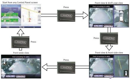
When the shift lever is in the R (REVERSE) position and the CAMERA button 1 is pressed, the following views will display in order:
