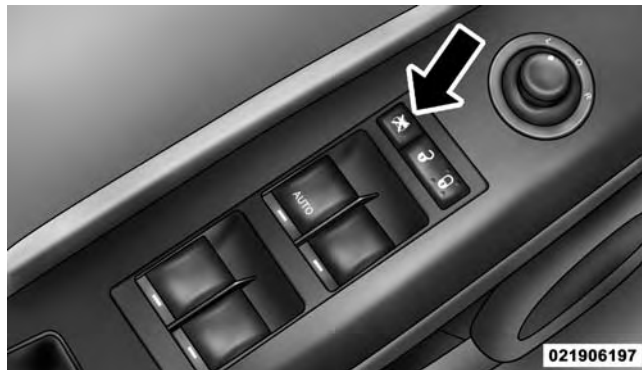
Window Lockout Switch
