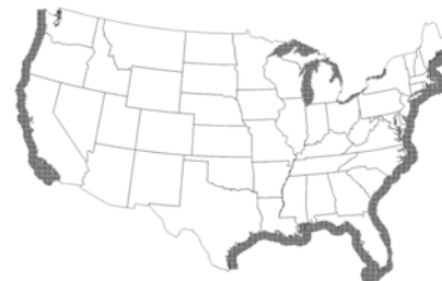
Using Openwind, 7,159-unit wind power plants were modeled throughout the resource area of the continental United States from 0 nautical miles (nm) to 50 nm
