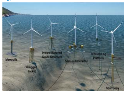
Offshore wind substructure types for varying water depths. Illustration by Josh Bauer, National Renewable Energy Laboratory
