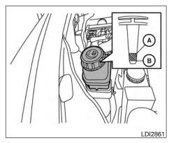
Check the fluid level in the reservoir.
