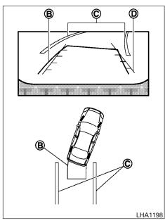
Slowly back up the vehicle adjusting the steering wheel so that the predicted course lines
