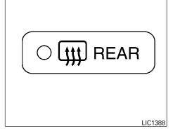
To defrost the rear window glass and outside mirrors (if so equipped), start the engine and push the rear window defroster switch on. The rear window defroster indicator light on the switch comes on. Push the switch again to turn the defroster off.
