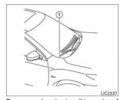
Be sure you do not put anything on top of the autolight sensor located in the top side of the instrument panel (1). The autolight sensor controls the autolight: if it is covered, the autolight sensor reacts as if it is dark out and the headlights will illuminate. If this occurs while parked with the engine off and the ignition switch placed in the ON position, your vehicle's battery could become discharged.
