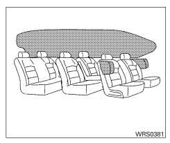
Front seat-mounted side-impact supplemental air bag and roofmounted curtain side-impact and rollover supplemental air bag systems
