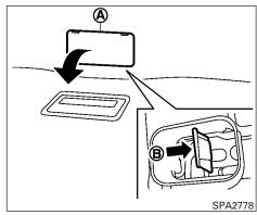
Manual liftgate release (if so equipped)
