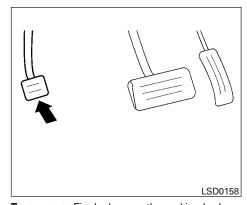
**To engage:** Firmly depress the parking brake.
