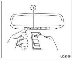
2. Using both hands, simultaneously press and hold the desired HomeLink® button and hand-held transmitter button. DO NOT release until the HomeLink® indicator light ① flashes slowly and then rapidly. When the indicator light flashes rapidly, both buttons may be released. (The rapid flashing indicates successful programming.)
