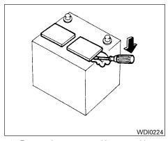
Remove the vent caps with a screwdriver as shown. Use a cloth to protect the battery case.
