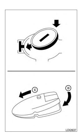
3. Replace the battery with a new one.
