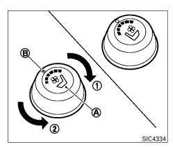
The climate controlled seat warms up or cools down the front seat by blowing warm or cool air from under the surface of the seat. The climate control switch is located on the center console.
