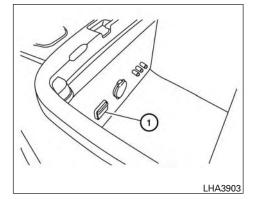
USB (Universal Serial Bus) CONNECTION PORT (models with Navigation System) (if so equipped)
