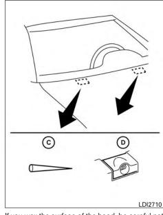
If you wax the surface of the hood, be careful not to let wax get into the washer nozzle ①. This may cause clogging or improper windshield-washer operation. If wax gets into the nozzle, remove it with a needle or small pin ②.
