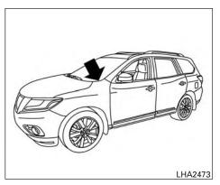
The sunload sensor, located on the top driver's side of the instrument panel, helps the system maintain a constant temperature. Do not put anything on or around this sensor.
