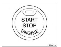
When the ignition switch is pushed without depressing the brake pedal, the ignition switch will illuminate.
