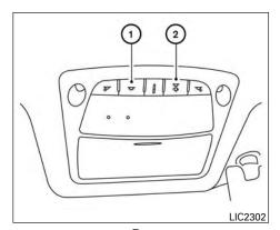
When the ON switch (1) is pressed, the footwell lights (if so equipped), step lights (if so equipped), map lights and rear personal lights will automatically turn on and stay on for a period of time when:
