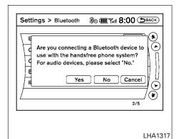
4. A screen will appear asking if you are connecting the device to use with the handsfree phone system. Select the "No" key.
