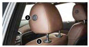
To raise the head restraint: Pull the head restraint up.
