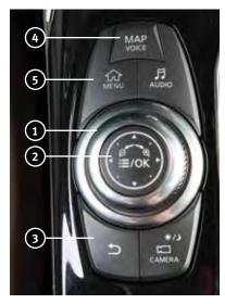
Use the Infiniti controller (1) and  $\mathbf{OK}$  button (2) to navigate through the center display screens.
