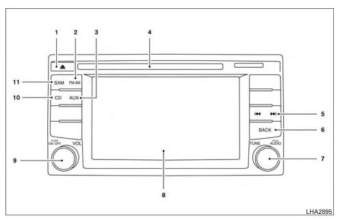
FM/AM/SAT RADIO WITH COMPACT DISC (CD) PLAYER (Type B) (if so equipped) For additional information, refer to "Audio operation precautions" regarding all operation precautions in this section.
