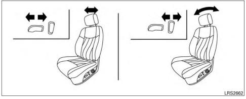
FRONT POWER SEAT ADJUSTMENT (if so equipped for driver's seat)
