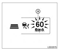
When passing another vehicle, the set speed indicator (B) will flash when the vehicle speed exceeds the set speed. The vehicle detect indicator will turn off when the area ahead of the vehicle is open. When the pedal is released, the vehicle will return to the previously set speed.
