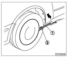
Removing wheel cover (if so equipped)
