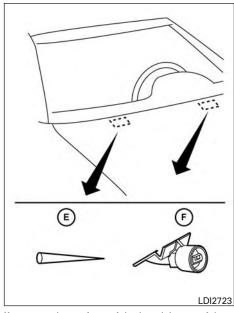
If you wax the surface of the hood, be careful not to let wax get into the washer nozzle (F). This may cause clogging or improper windshield-washer operation. If wax gets into the nozzle, remove it with a needle or small pin (E).
