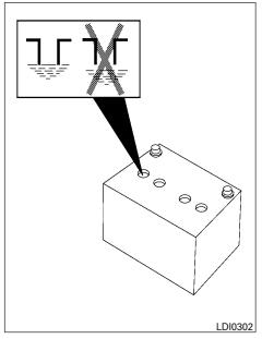
Check the fluid level in each cell. If it is necessary to add fluid, add only distilled water to bring the level up to the bottom of the filler opening. Do not overfill. Reinstall the vent caps. Vehicles operated in high temperatures or under severe conditions require frequent checks of the battery fluid level.
