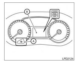
LOOSE FUEL CAP warning message For vehicles without a vehicle information display: Push the reset button (a) for more than 1 second to reset the LOOSE FUEL CAP warning message in the trip computer (b) after the fuel cap has been tightened. For additional information, refer to "Fuel-filler cap" in the "Pre-driving checks and adjustments" section of this manual.
