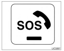
The E-call (SOS) system switch is used in combination with a NissanConnect SM Services subscription to call for assistance in case of an emergency.
