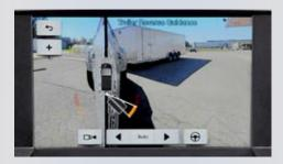
Utilizes 3 cameras to provide multiple views along with steering guidance graphics to assist in backing and manoeuvring a trailer
