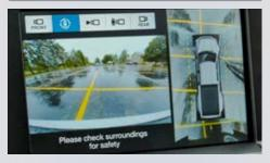
Trailer Reverse Guidance uses 3 cameras to provide multiple views of trailers, as well as steering guidance graphics, to assist with trailer manoeuvres while in reverse
