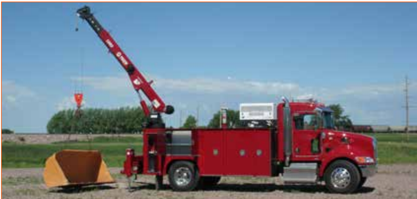
The 1069 Tiger Crane features 29 ft of hydraulic reach and 11,000 lbs of lifting capacity, all in a crane that can be mounted on a 25.5k GVW or larger chassis.
