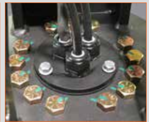
Sealed Center Rotation eliminates the need for a drip pan in the crane tower.
