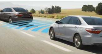
**PRE-COLLISION SYSTEM<sup>11</sup>** The available Pre-Collision System<sup>11</sup> uses radar to help determine if a frontal collision is imminent.
